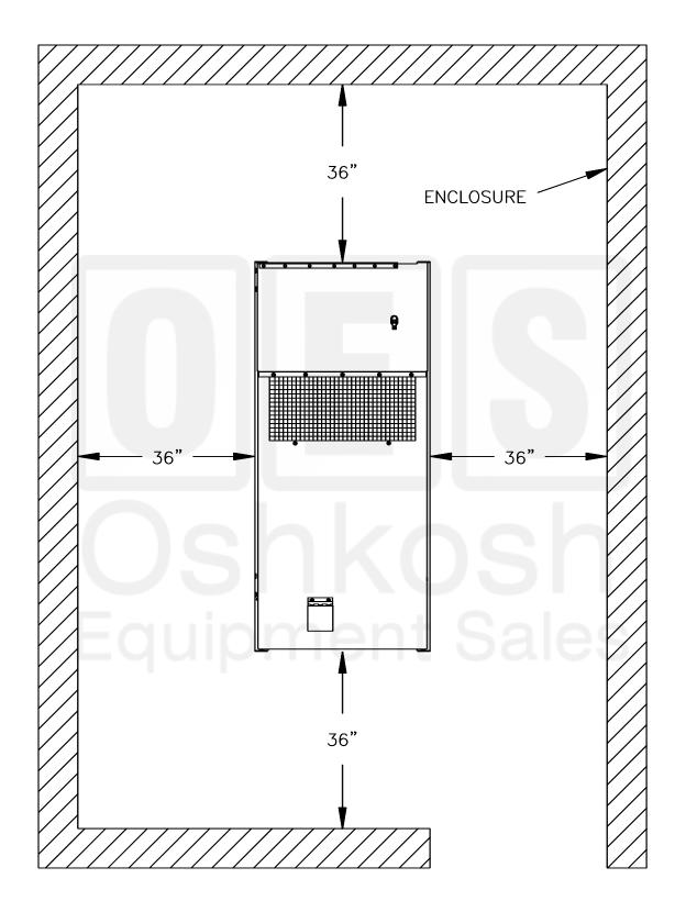
FIGURE 2-5. MINIMUM ENCLOSURE CLEARANCE MEASUREMENTS
